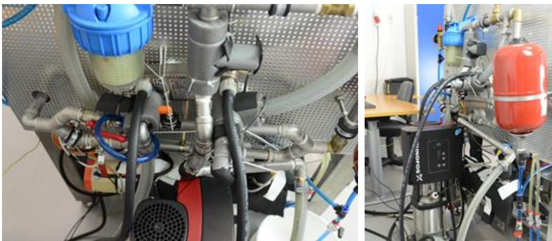
Fig. 4.1. Flow system of the magnetocaloric heat pump developed at DTU Energy
