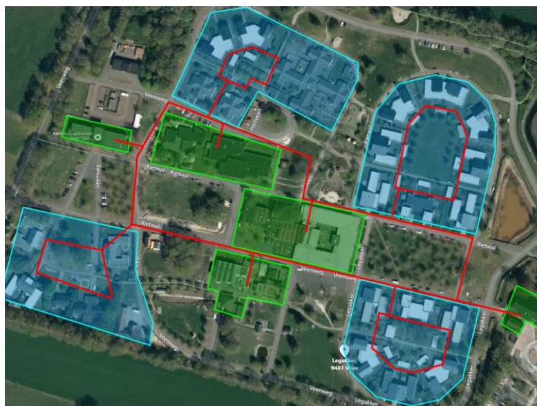
Figure A-10-6: IES solution Vries site (red = heating/cooling grid connected to all buildings)
