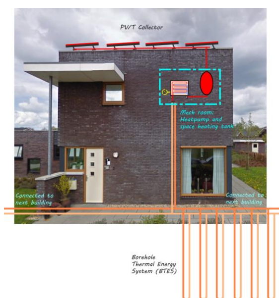
Figure A-10-4: Suggested implementation of water/water heat pump, PV/T collectors and BTES per building block
