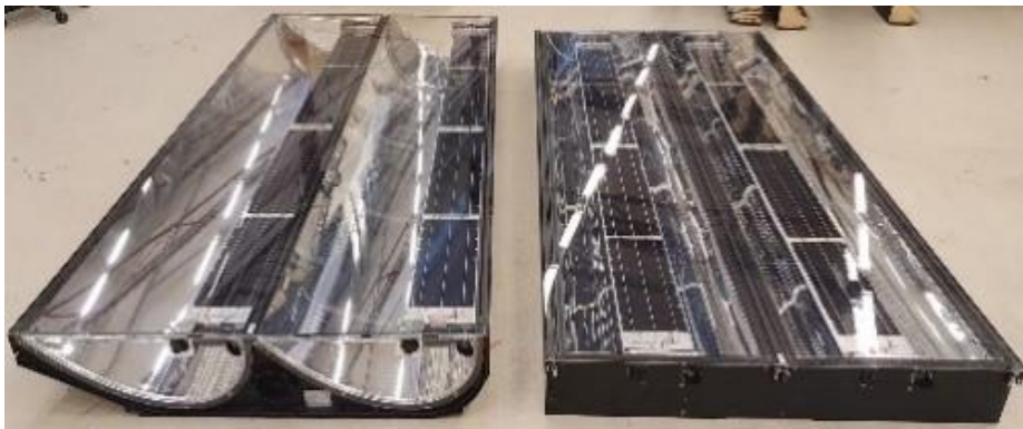
Figure A-9-3: PV/T Collector
