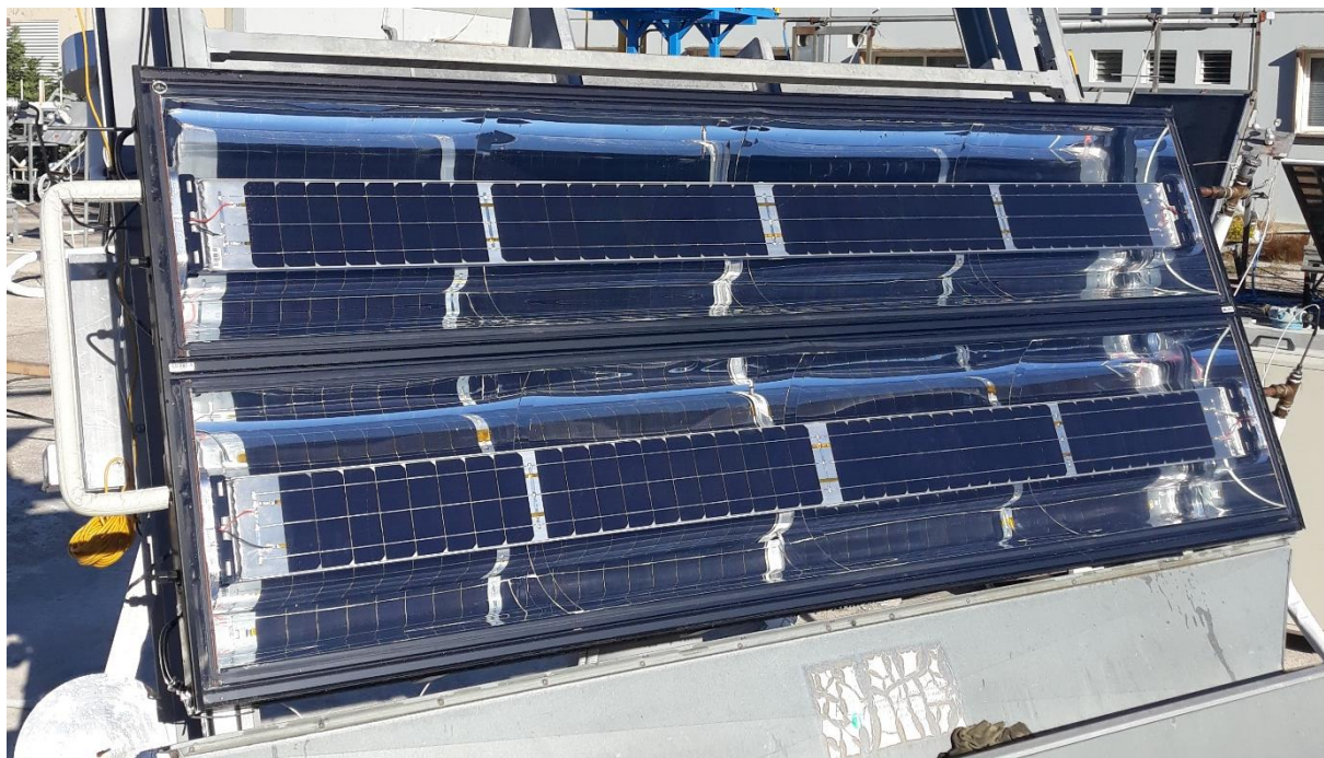
Image caption: The prototype PVT collectors with novel reflector geometry undergoing testing in Greece ©NCSR Demokritos
