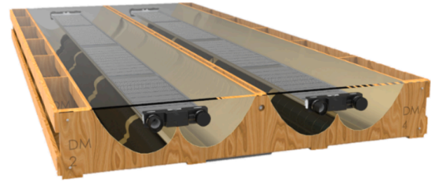
Fig. 5. CPVT collector comprising two geometries (CPC 1 and 2) with identical PVT receivers (PV cell string configuration of 8-11-11-8 PV cells).
