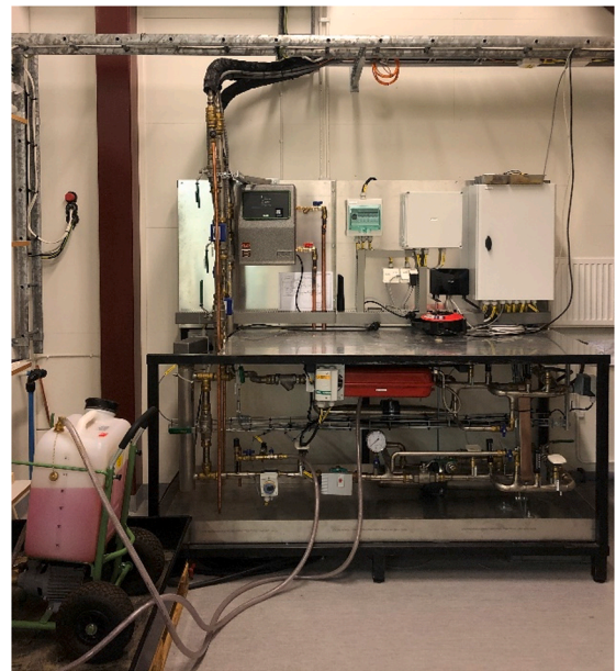
Fig. 7. Thermal test rig design to cope with the specifications of ISO 9806:2017 testing procedure with an auxiliary pump station.
