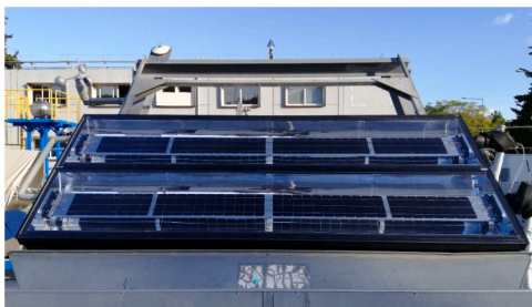
Fig. 3. PVT collector mounted at the tracker and charged with water/glycol.
