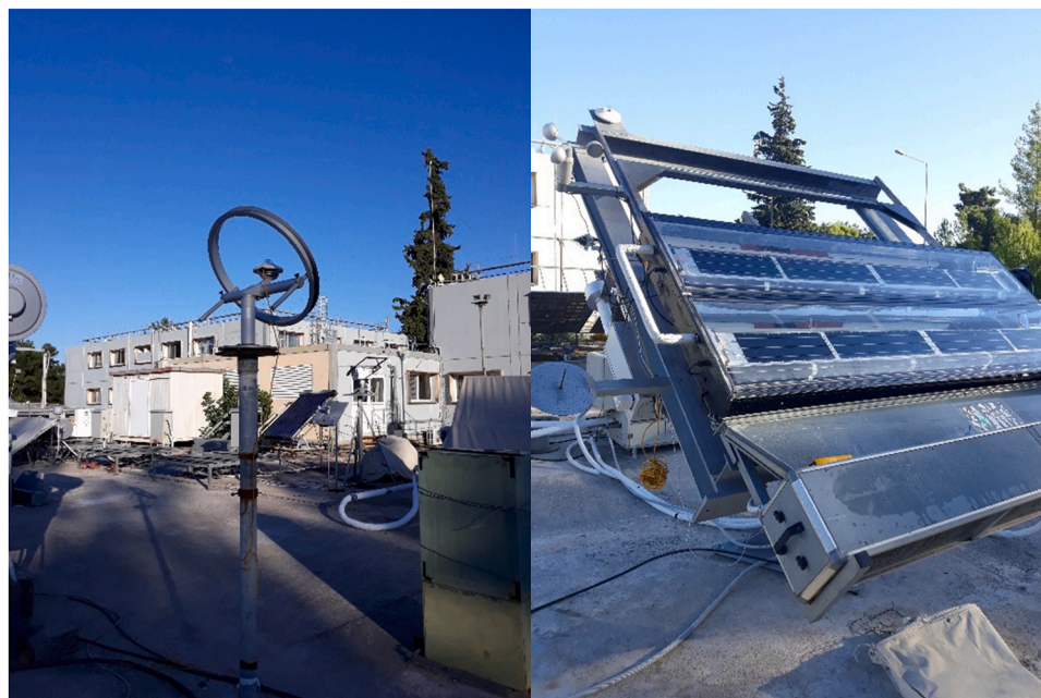
Fig. 4. Left: Pyranometer for diffuse radiation placed next to the stand. Right: Testing of the collector started early in the morning.
