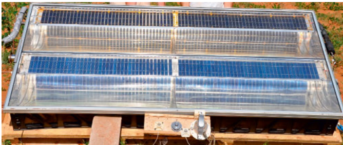
Figure 71. Detailed view of the C-PVT V1 and the pyranometers
