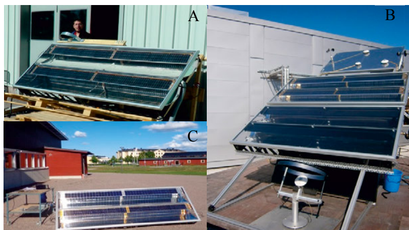
Figure 80. Outdoor measuring for Paper IV: (a) Solarus Factory PVT V2; (b) Dalarna University PVT V3; (c) Gävle University PVT V4.
