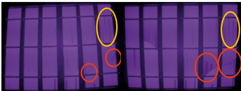
Figure 44. EL test of receiver 5. (A) Baseline (ambient temperature); (B) After the round at 200 °C.
