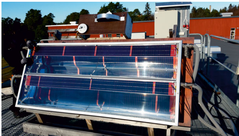
Figure 91. Early collector stand at HiG with the two pyranometers.
