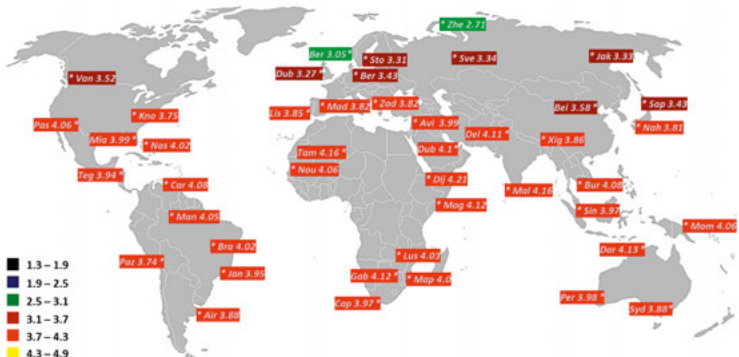
Figure 40. Ratio Vacuum tube with flat absorber 50 °C to PV monocrystalline [1].
