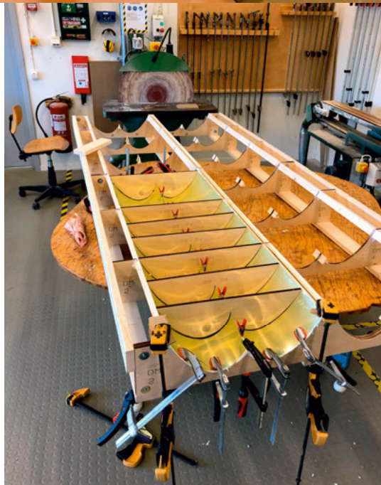
Figure 134. Two steps of the construction process of the DM C-PVT collector.
