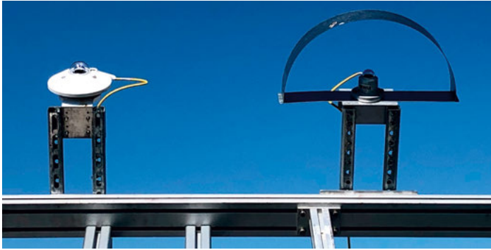
Figure 141. CMP3 and CMP6 solar radiation sensors for both global and diffuse radiation, respectively.
