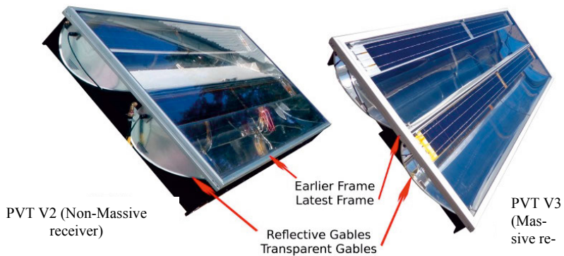
Figure 82. Differences between PVT V2 and PVT V3.
