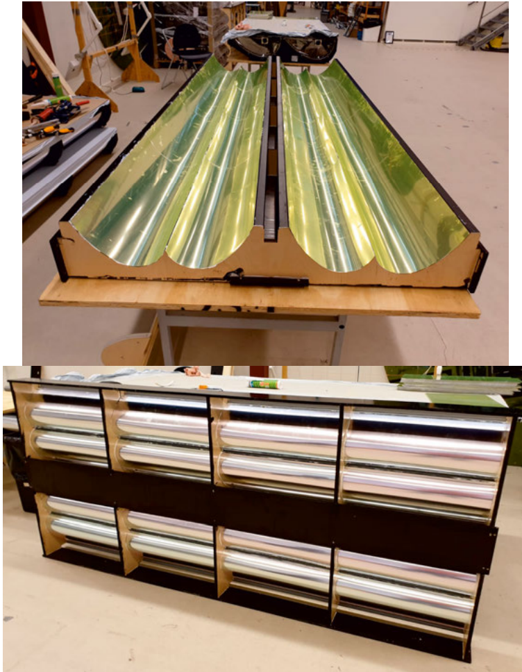
Figure 136. Two steps of the construction process of the DM C-PVT collector.
